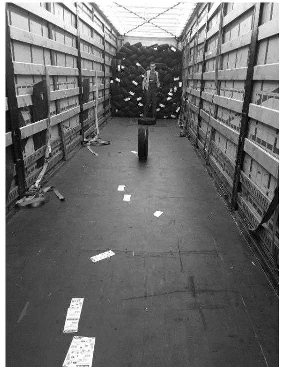
Fig. 2. The method of rolling tires from a tractor unit.
