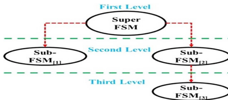
Fig. 6. Stack layers of HGFSM
