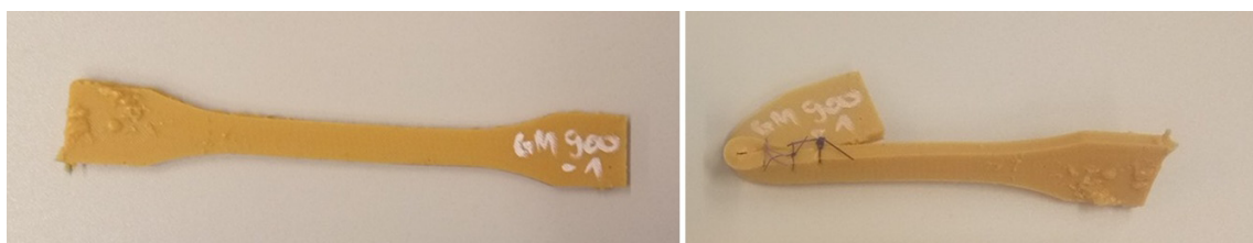
Fig. 5. Resin samples before (left) and after (right) suturing
