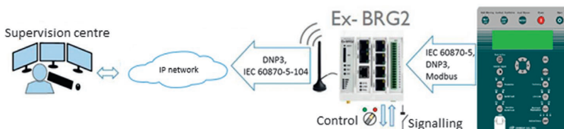
Fig. 6. Functional diagram of communication between the KTR 27 recloser and supervision centre [11]
