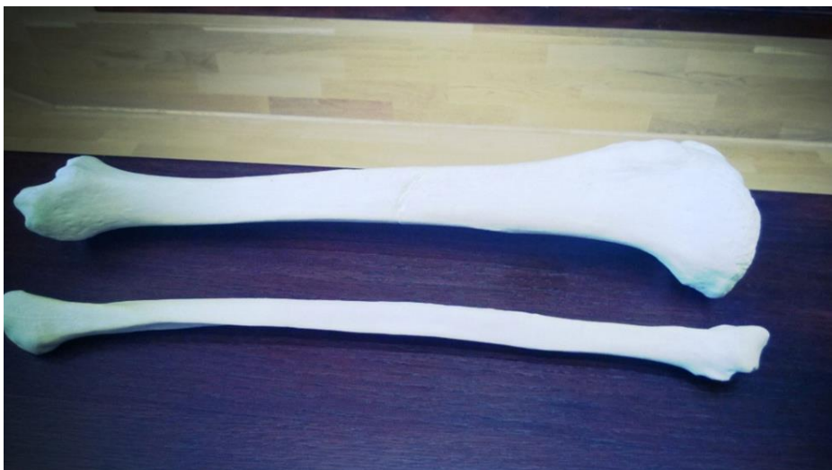
Fig. 4. 3D print of spatially scanned human bones
