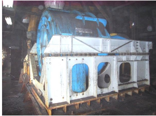
Fig. 3. WOK 1.5 centrifuge in sound-insulating enclosure [7]
