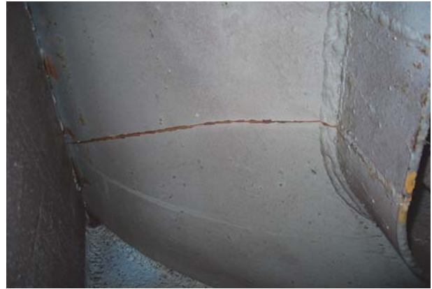
Fig. 6. Crack of the short support tube buffet – at app. 1/3 of a perimeter
