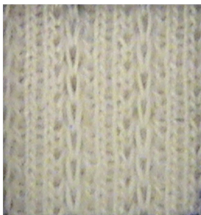
Figure 1. Some knitted pattern examples formed by tuck stitches [3].
