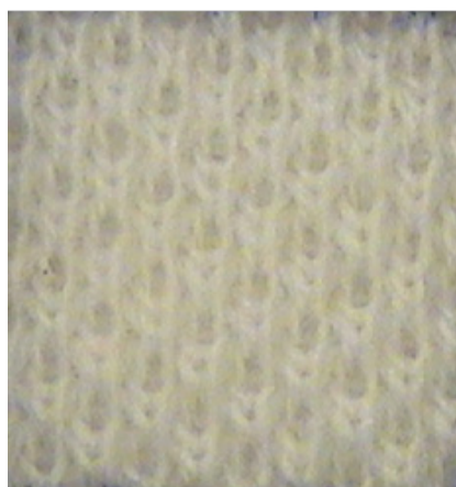
Figure 1. Some knitted pattern examples formed by tuck stitches [3].
