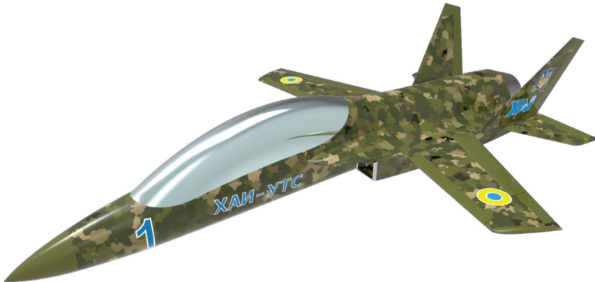
Fig. 11. Master geometry of the jet training aircraft.
