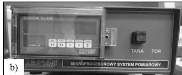
Fig. 2. Test apparatus – pin-on-disc station and force measurement system: a) Pin-on-disc station, b) Friction force measurement system [L. 5]
