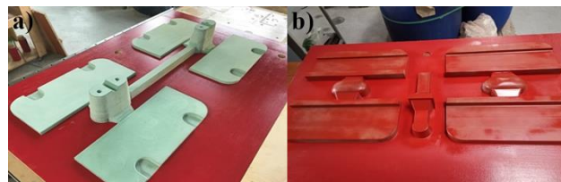
Fig. 7. Molding in OMEGA device: a) upper model plate for molding; b) bottom plate for the molding
