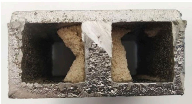
Fig. 12. Test casting after core discharge
