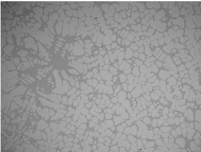
Fig. 18. Microstructure of the sample cast under pressure with value 150 MPa, zoom 100x, etching 0.5% HF
