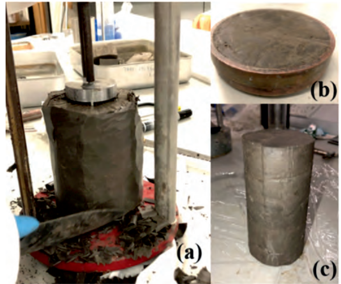
Fig. 2. (a) Sample trimming, (b) specimen for oedometer test and (c) specimen for triaxial test
