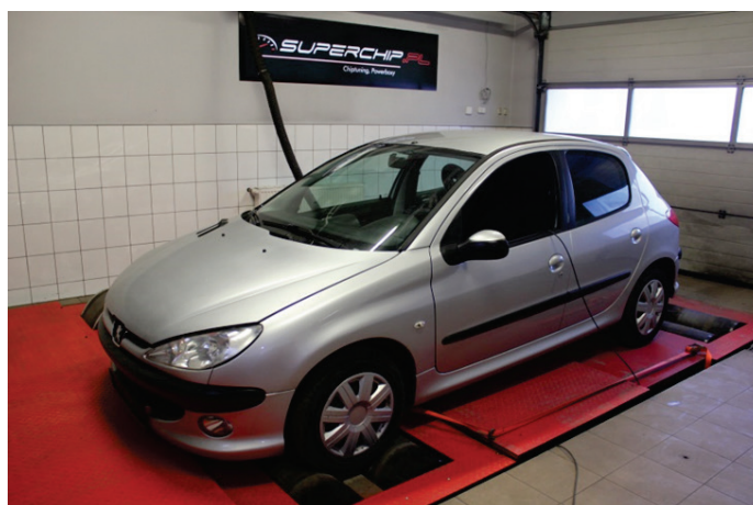
Fig. 2. View of the tested vehicle on the chassis test bed
