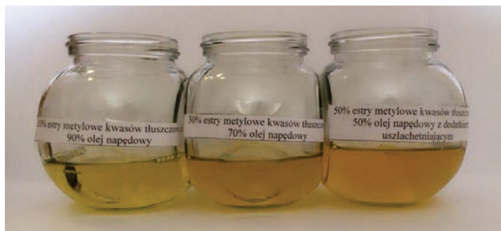
Fig. 1. Mixtures of diesel oil and the fatty acid methyl esters
