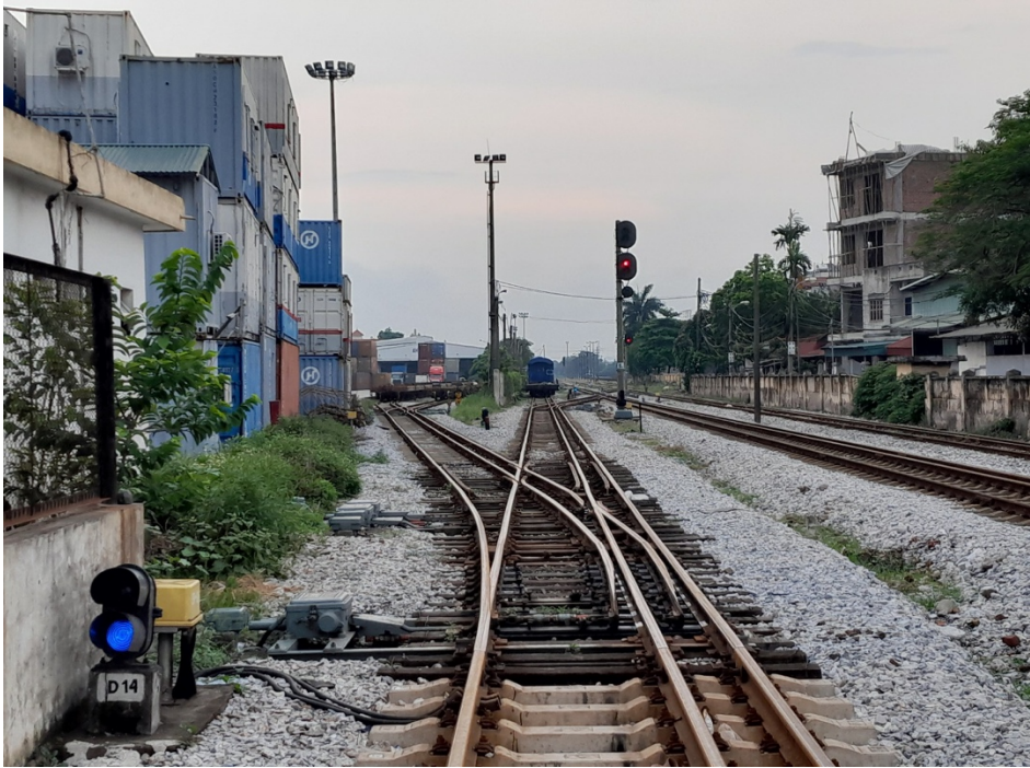
Fig. 5. One of the many loading points (here: with an additional track for handling containers) in the area of the Yên Viên station where an infrastructure based on two track gauges is used. June 6, 2023
