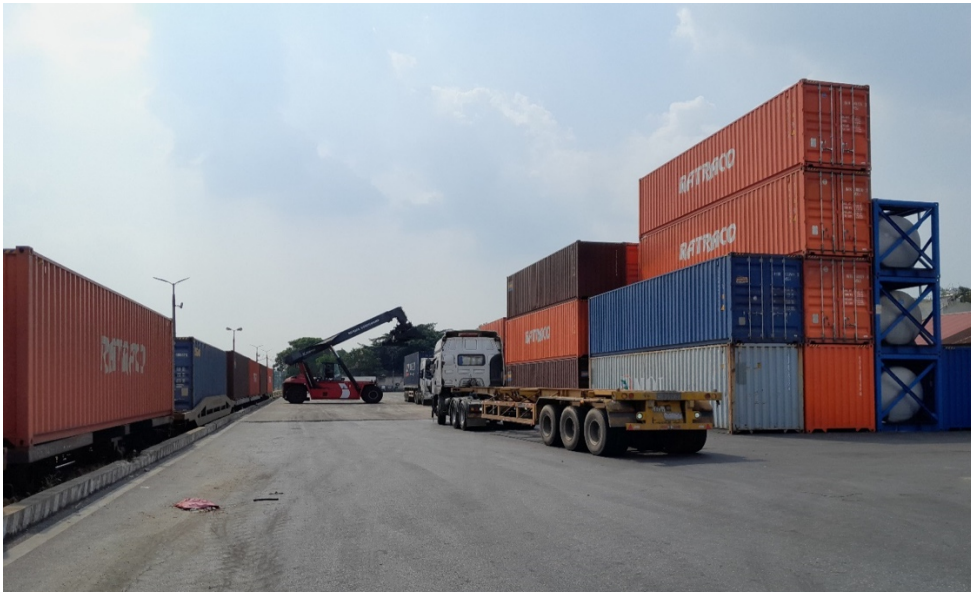
Fig. 6. Container terminal at Đông Anh station (northeast Hanoi) after the arrival of the container train from China (flatcars are located on the gantlet track 1,000-1,435 mm). June 11, 2023
