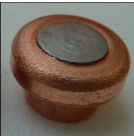
Fig. 17. Comparison of concave head element with the simulation of die cavity filling
