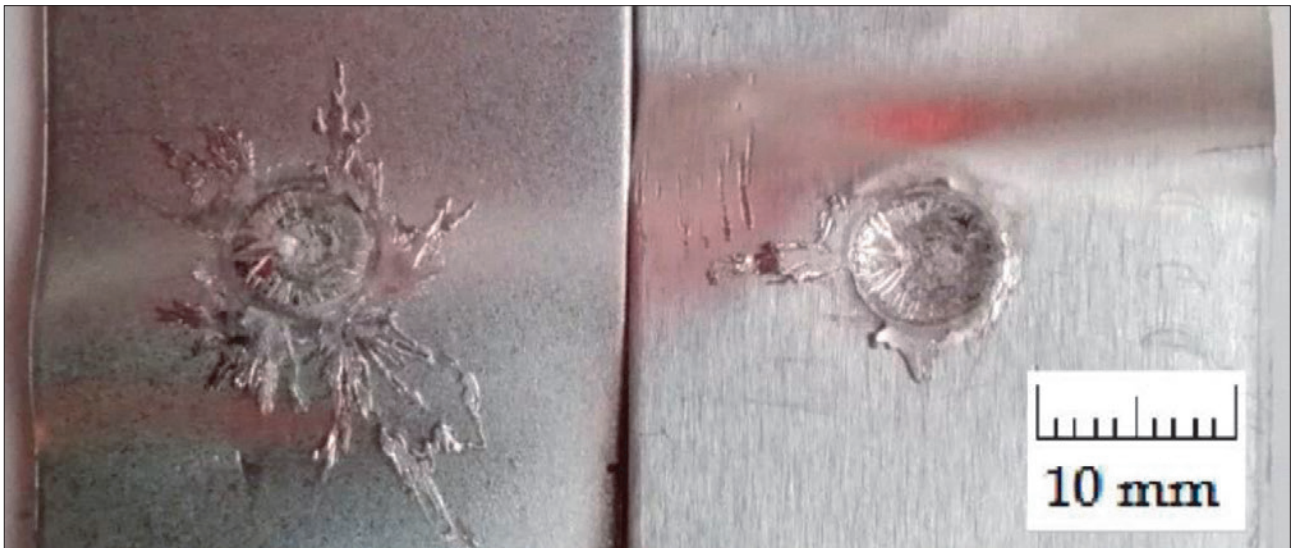
Fig. 2. Splash formation in the REW technology
