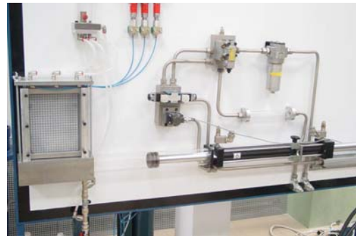
Fig. 1. View of the stand for analysis of the flow phenomena occurring during research of filling the model mould [12]
