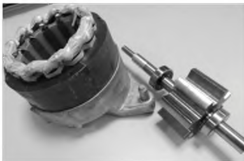
Fig. 2. Stator and rotor of SRM made from powdered material
