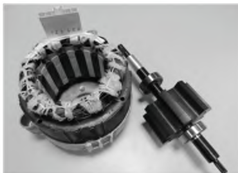
Fig. 1. Stator and rotor of conventional SRM model
