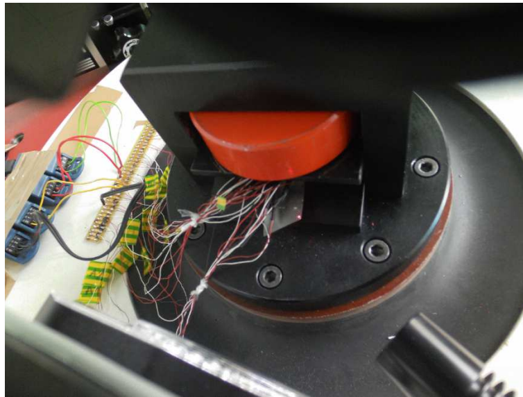
Fig. 8. Blade in a hydraulic holder mounted on the electrodynamic shaker
