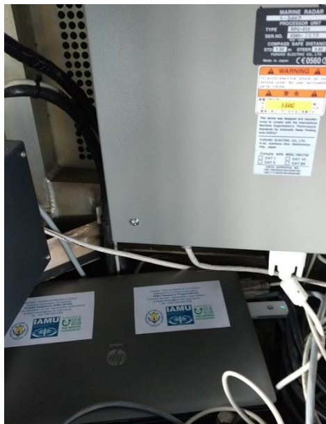
Figure 2. A system for navigational data registration.
