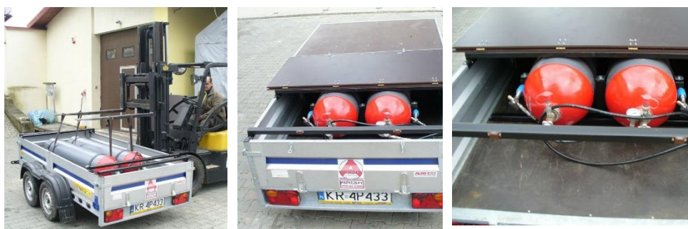
Figure 7. View of the transport trailer with biomethane cylinders, secured on the trailer.
