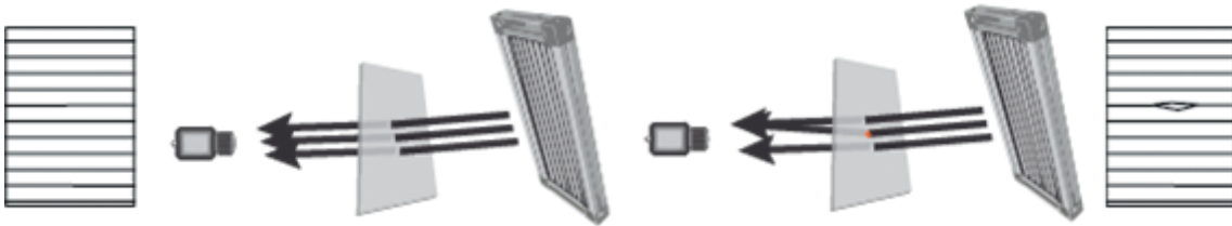
Fig. 3. Transparent objects and phase measuring deflectometry [3]
