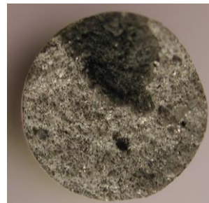
Fig. 5. The fracture surfaces of the tensile specimens with large Y_2O_3 inclusion (dark color). Identification of Y_2O_3 was performed by XRD and SEM-EDS analysis. The diameter of specimen is 6 mm
