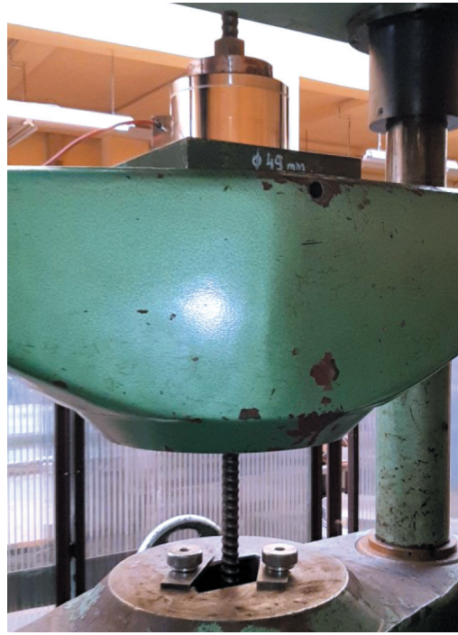
Fig. 12. Anchor rod mounted in a fatigue testing machine
