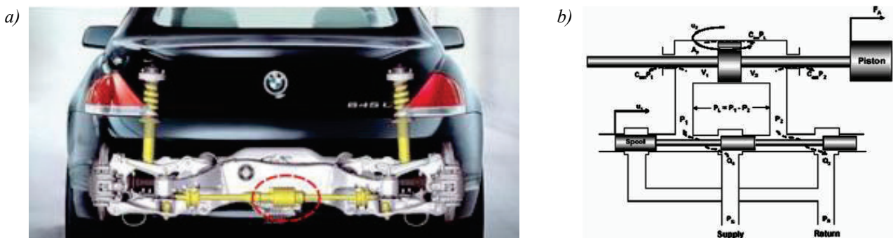
Fig. 4. BMW active anti roll control: a) BMW hydraulic active suspensions [2], b) hydraulic actuator schematic [2]
