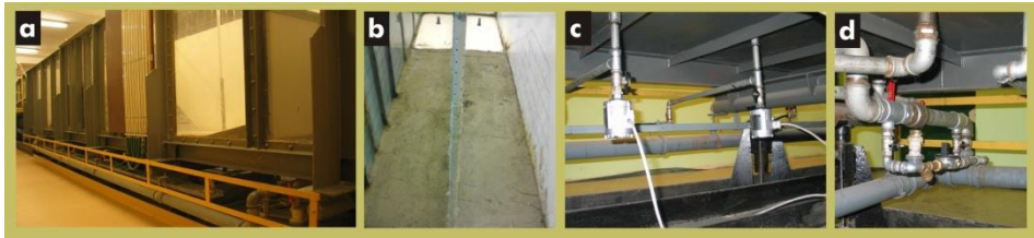
Fig. 1. Medium size apparatus for testing filtration through model embankments: a) a headwall view, b) the inside of the apparatus with the clayey bottom sealing, c) pressure transmitters for measurements of water level, d) measurement-and-spillway valves
