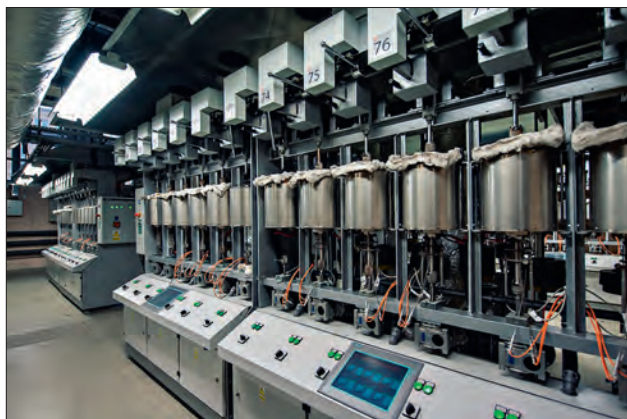
Fig. 2. Six-stand single-sample machines for creep tests manufactured by IMŻ
