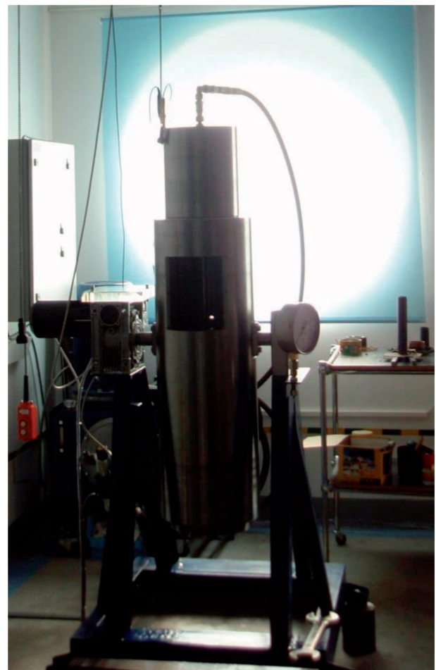
Fig. 3. Press for cold hydrostatic extrusion under a pressure up to 2.5GPa (designed and constructed at Unipress)
