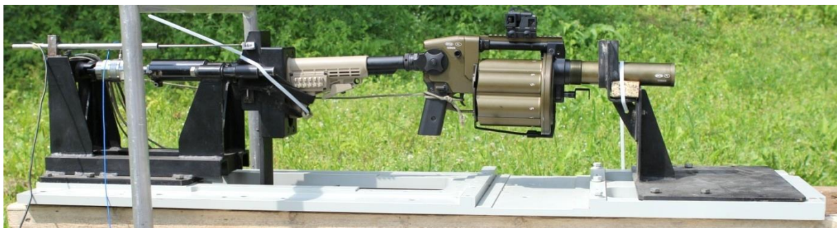
Fot. 4. Granatnik RGP-40 na stanowisku badawczym strzeleckim 4012.0.1.S100 Photograph 4. Grenade launcher RGP-40 on the firing testing stand No 4012.0.1.S100
