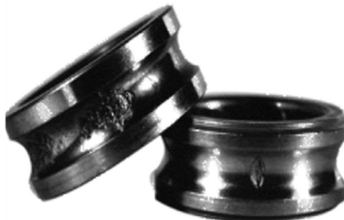
Fig.2. Inner ring with defect [28].
