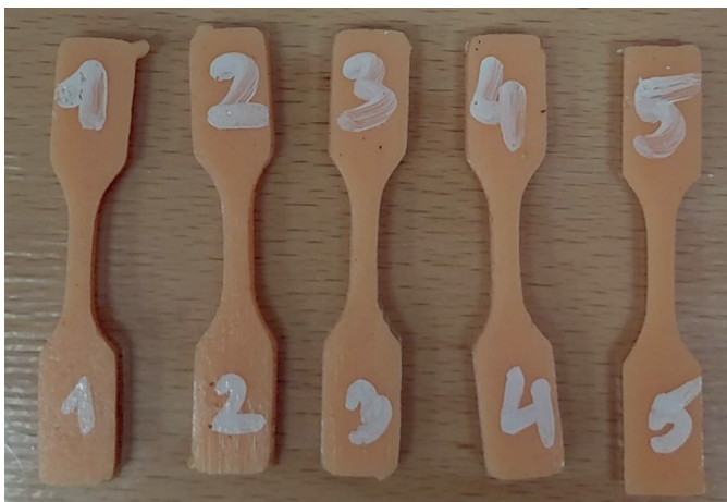
Fig. 2. Tensile testing samples: reference material (a) and drug-silicone composite (b)
