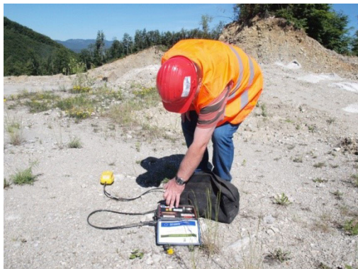
Figure 8. Standpoint – S1 and localisation of digital seismograph VMS 2000 MP and seismic receivers by Geospace located 18.6 m away from the first initiated borehole of the blast I. in the quarry Lopušné Pažite
