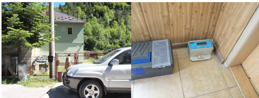
Figure 9. Standpoint – S2 with seismographs ABEM Vibraloc and seismic receivers ABEM installed in the distance of 241 m from the first blast I. and in the distance 246 m from the second blast II. in the village Lopušné Pažite
