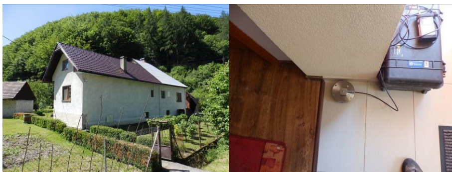
Figure 10. Standpoint – S9 with seismographs SvanteK and seismic receivers SvanteK installed in the distance of 311 m from the first blast I. and in the distance of 309 m from the second blast II. in the village Lopušné Pažite
