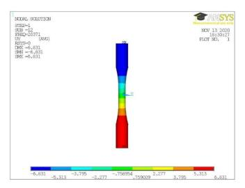
**Fig. 3.** Axial  $(u_x)$  displacements for the basic frequency mode
