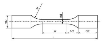
Fig. 1. Geometry of the analysed elements (cross-section)
