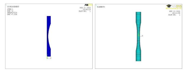
Fig. 2. FEM mesh of axisymmetric model in Ansys: plane (left), spatial (right)
