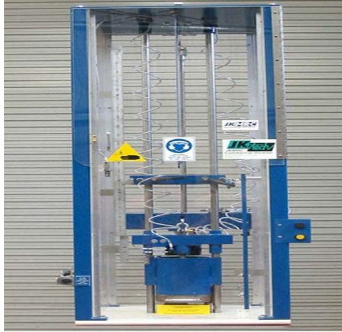
Fig. 1. Drop-weight test apparatus
