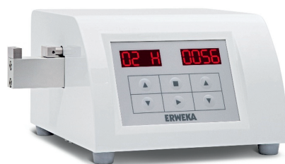
Fig. 3. Erweka GmbH for measuring the compressive strength of fertilizer granules
