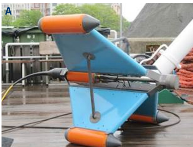
Fig. 1. a) Magnetometr SeaQuest by MarineMagnetics (Canada)(fot. W. Konieczny); b) Magnetometr by Geometrics (USA) (source: www.geometrics.com)
