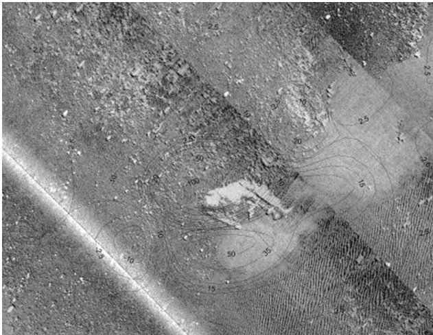
Fig. 4. Side scan sonar image of the shipwreck in detected magnetic anomaly PIIB-AM001 (Gulf of Koszalin)
