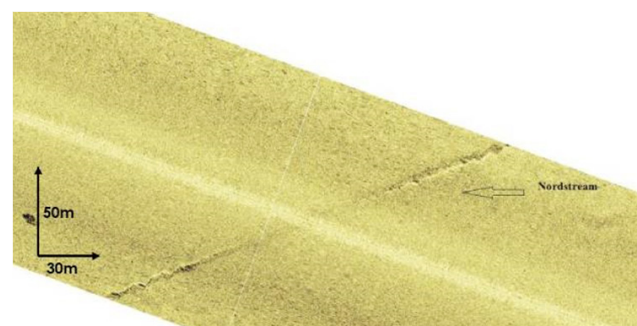
Fig. 11. Side Scan Sonar image at the site of North Stream gas pipeline
