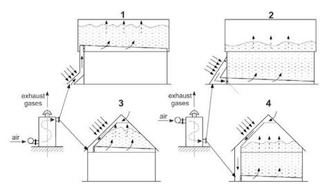
Figure 6. The principle of cooperation of a heating unit with dryers equipped with solar collectors in an attic and in a barn: 1, 2 – wall collectors; 3, 4 – under-roof collectors Source: authors' own work.
