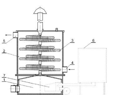
**Figure 7.** The air heater equipped with biomass stove: 1 – combustion chamber, 2 – heat exchanger, 3 – tubular section of flue, 4 – air inlet, 5 – air outlet, 6 – biomass heating unit with biomass-storage cell, 7 – burner
