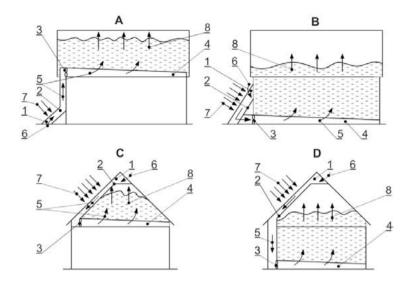
Figure 4. Basic rules for installing solar collectors in farm buildings; A – wall collector with drying room in the loft, B – wall collector with dryer in the barn, C – under floor collector with drying room in the loft, D – under roof collector with drying room in the barn: 1 – air inlet, 2 – collector, 3 – fan, 4 – distribution channel, 5 – heated air, 6 – ambient air, 7 – solar radiation, 8 – humid air
