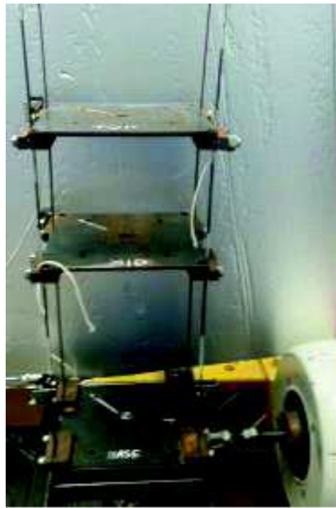
Figure 1. Time-variant three-floor building model
