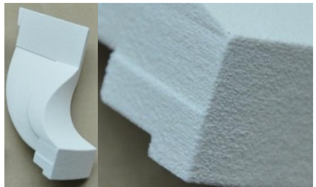
Fig. 3. Printed segment tooling with visible layers print
