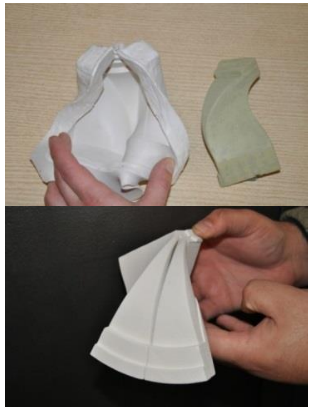
Fig. 5. Silicone matrix and removed out the model and a two assembly models together.
