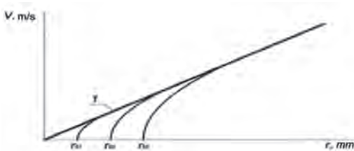
Fig. 2. Scheme of particle velocity change along the rotor blade at different values of the initial particle position ( r_{01} , r_{02} , r_{03} – the distance from the rotor centre to the starting points of the particle movement); 1 – asymptote of particle velocity
