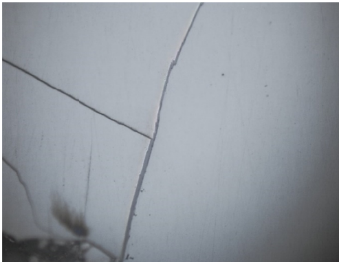
Picture 1. A cracked fragment of vitrinite-colotelinite, coal seam 406/1, magnification 500×, reflected light, immersion
