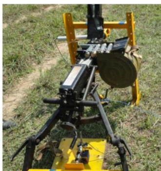
Fig. 6. Experimental way of stability investigation: 1 – special frame system; 2, 3 – displacement transducers DTH-A-100; 4 – measuring mount.
