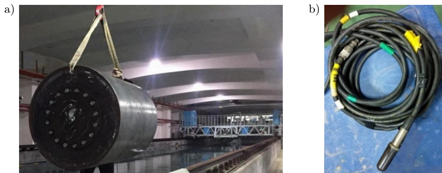
Fig. 3. Photograph of the watertight steel circular cylindrical shell being loaded into the towing tank (a) and the B&K 8104 hydrophone used to measure underwater noise (b).
