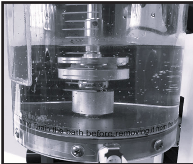
FIG. 3. Test stand for endurance tests, with the temporomandibular joint disc preparation to be tested, in holding wraps, in a saline bath at 37.5°C.
