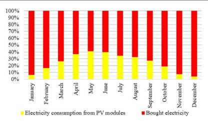
Fig. 4. Distribution of the electricity consumption on the Jasmini Farm in 2020 (*own research*)
