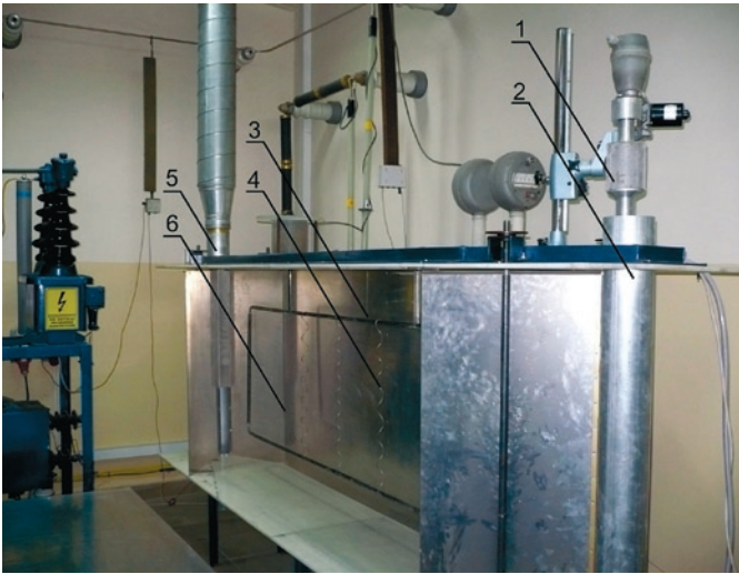
Fig. 4. View of laboratory electrostatic precipitator with removed collecting electrode. 1 – the dust feed system, 2 – diffuser, 3 – frame of discharge electrodes, 4 – discharge electrode, 5 – confusor; 6 – collecting electrode
