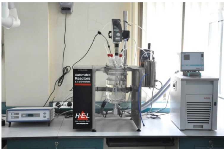
Figure 2. Laboratory scale facility used for t-GAP process optimization
