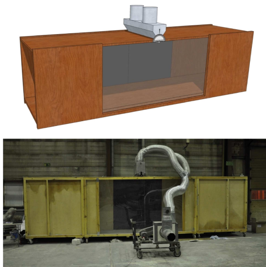
Fig. 8. Scheme (up) and a photograph (down) of the test tunnel facility (Ref. 19)
