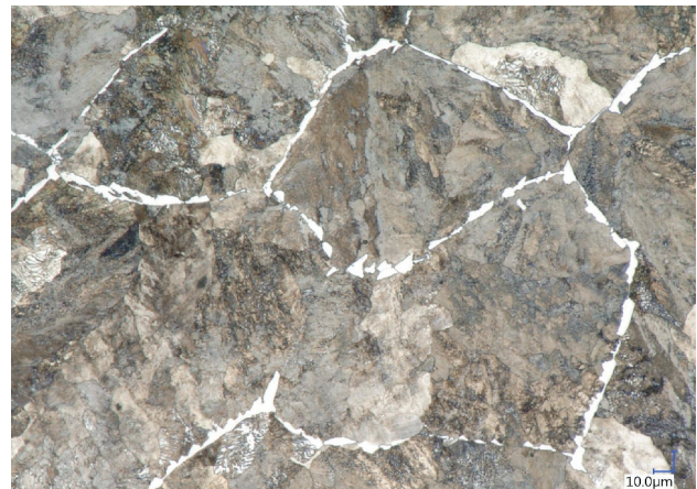
Fig. 15. Flash-butt welding line of the rail joint of the grade R260 after fatigue tests [authors' own photo]
