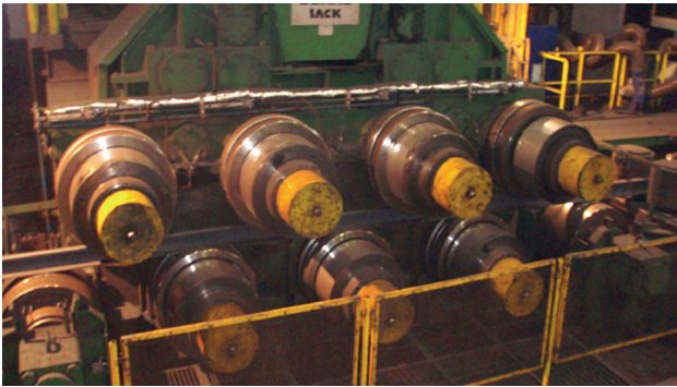
Fig. 2. Rails straightening in a nine-roller straightener [authors' own photo]
