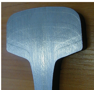
Fig. 3. Cross-section of the rail head after cutting with a saw blade [authors' own photo]
