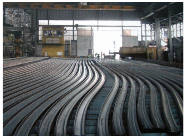
Fig. 1. Cooling of the rails after rolling on the cooling bed [authors' own photo]
