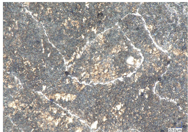
Fig. 16. Flash-butt welding line of the rail joint of the grade R350HT after fatigue tests [authors' own photo]
